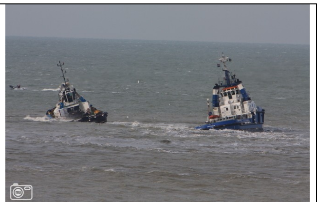
Towing on fixed object. Self tripping
