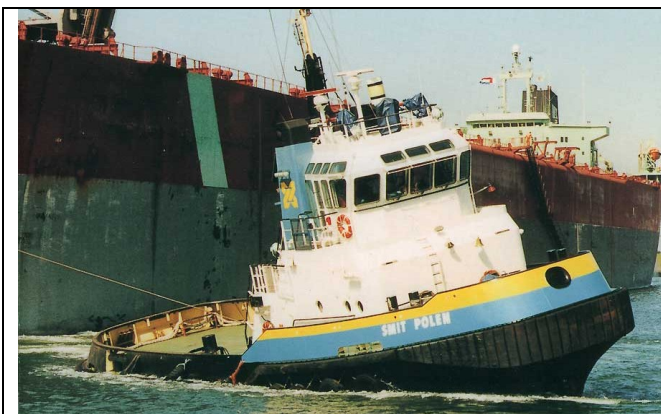
Towed by the tow: Tow tripping . Speed of tow and breaking load of towline are decisive.
