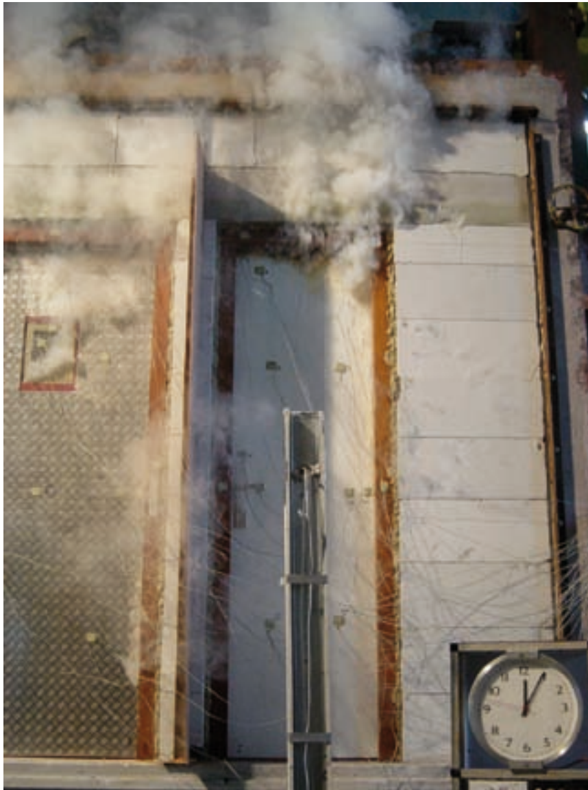
Figure 2: Smoke passing through the cell door and the door of the technical shaft, five minutes after the start of the test
